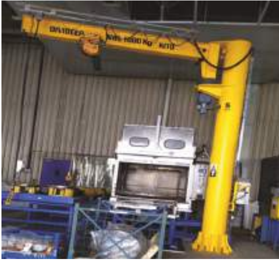
JIB CRANE WITH HOIST
