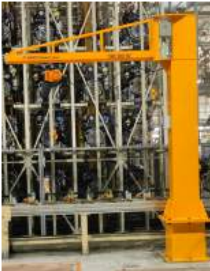
JIB CRANE WITH HOIST
