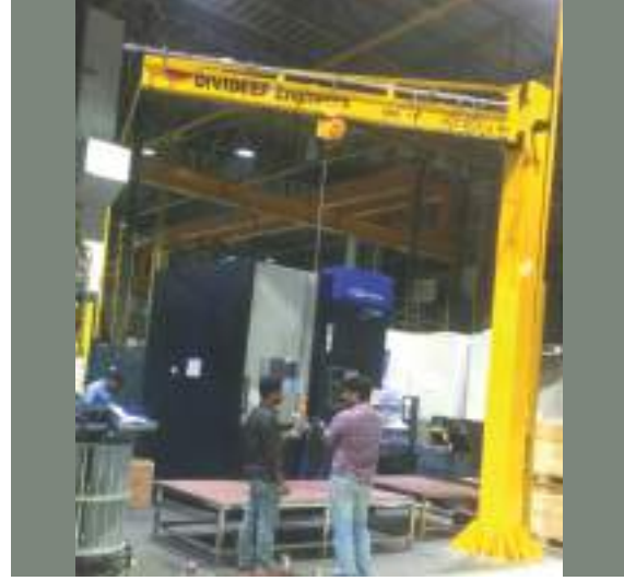
JIB CRANE WITH HOIST
